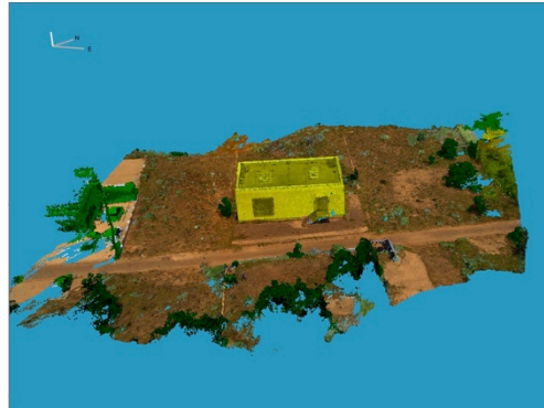
Building 3D model for damage survey with UAV
